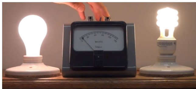
Figure 1. Compact fluorescent bulbs like the one on the right use a fraction of the energy of incandescent bulbs like the one on the left. Both bulbs shown here are 60 watt equivalent, yet the CFL uses only about 18 watts.
