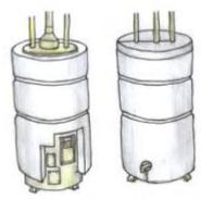
Most older water heaters have only an inch of fiberglass tank insulation, and most newer ones have just an inch of foam insulation. You can reduce your energy consumption by installing an additional blanket of fiberglass insulation. This is one of the most common and effective energy-conservation measures available.
